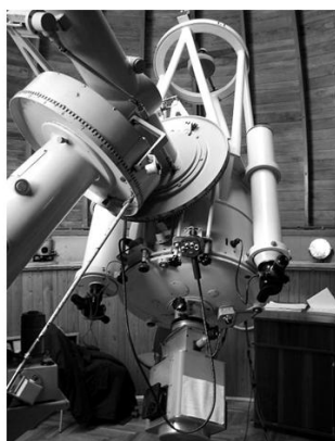
Figure 9: Two views of the 50cm Cassegrain telescope. Main features: Manufacturer: Carl Zeiss Jena; Year of installation: 1966; Focal length: 7500 mm
