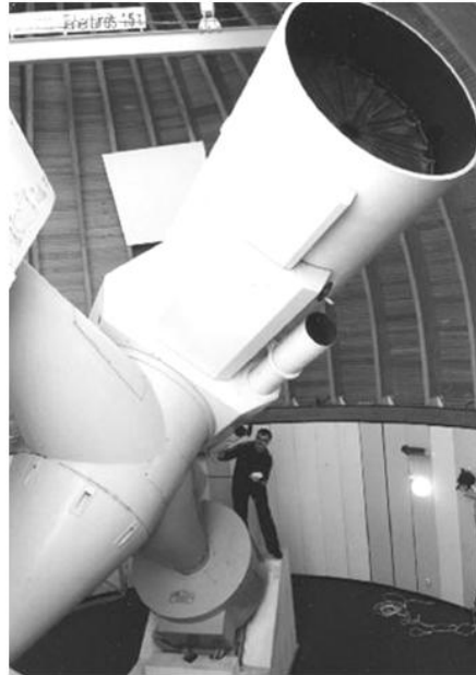
Figure 12: The 1 m RCC telescope. Main features: Manufacturer: Carl Zeiss Jena; Year of installation: 1974; Focal length: 13500 mm
