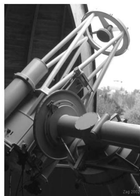
Figure 9: Two views of the 50cm Cassegrain telescope. Main features: Manufacturer: Carl Zeiss Jena; Year of installation: 1966; Focal length: 7500 mm
